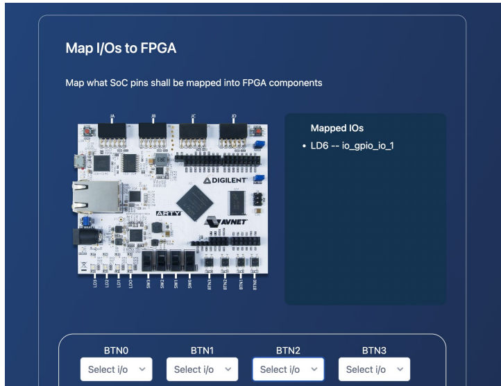
Mapping SoC IOs to FPGA Components
