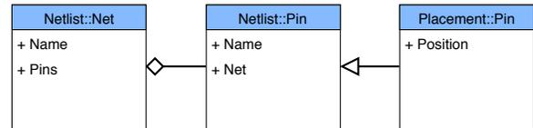
Figure 2: Class diagram representing a physical design problem with OOD approach. The diamond-end arrow between pin and net classes represents an aggregation relationship between two classes. The triangle-end arrow between the two pin classes represents a specialization relationship.
