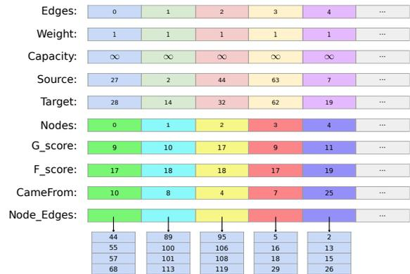
**Figure 5: Graph representation using DOD programming model.**
